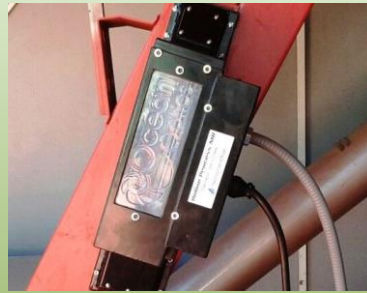
On-Line Sensor in the Combine Grain Elevation
